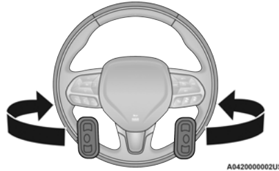
Remote Sound System Controls
